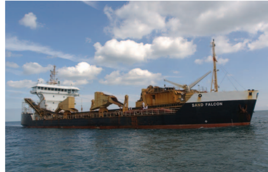
RMC Marine's Sand Falcon has been adapted to allow her to dredge to a depth of 50 metres
