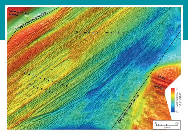
Seabed monitoring data for aggregate extraction area 351, 12 km east of the Isle of Wight, showing the results of a high resolution bathymetric survey over dredged seabed. There are over three million data points spaced just 0.5 metres apart recording water depths within the area shown. Criss-
