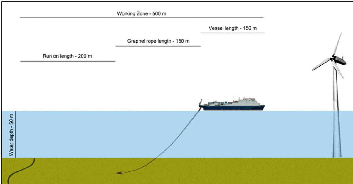
Figure 2 – Indicative distances required within the Working Zone when conducting cable recovery with grapnels in 50m depth of water (SCUK Guideline No 6 2012)
