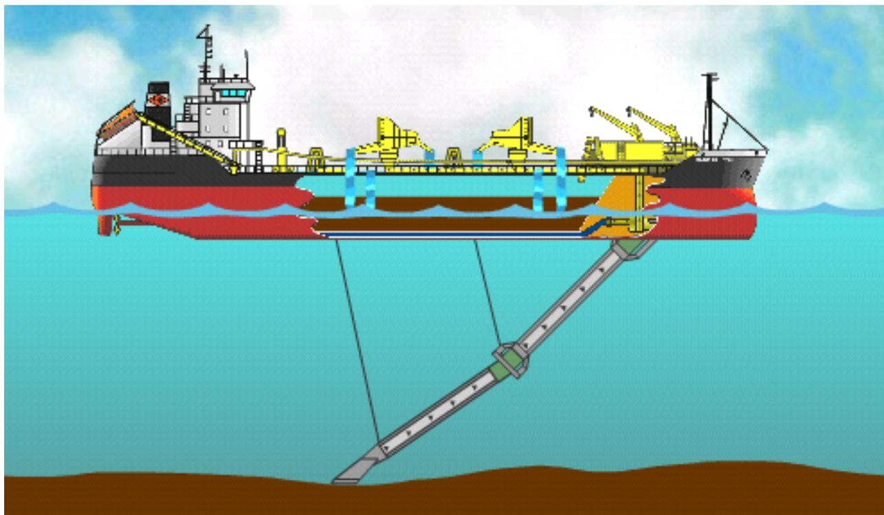
**Figure 5 - A Typical Trailing Suction Hopper Dredger**
