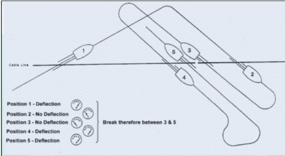
Figure 1 – The process of determining fault location through the use of trailed electrodes. (Internal Document, GMSL, 2011)
