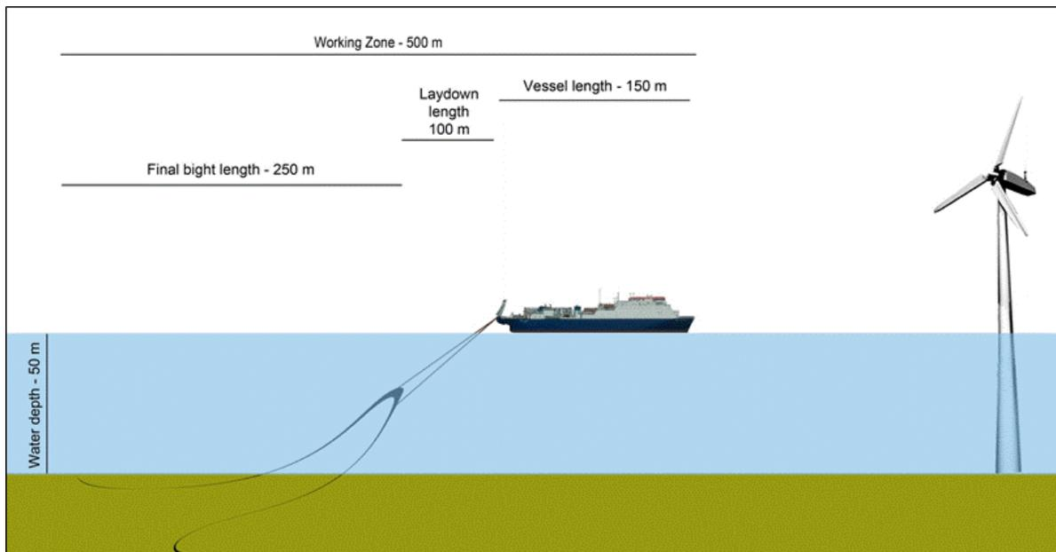
**Figure 3 – Indicative distances of cable line within the Working Zone when deploying a final bight to the seabed in 50m depth of water**
