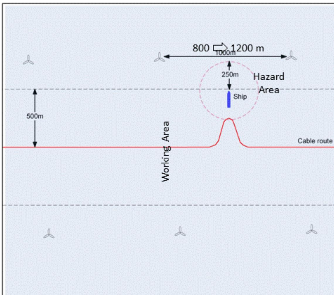
**Figure 4 - Vessel operation on the extent of the Working Zone when deploying a final bight**
