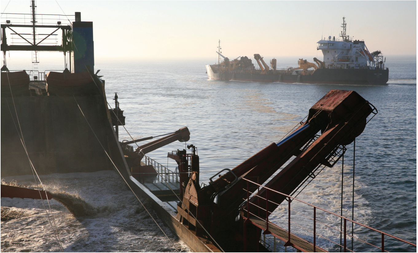
Figure 2. Two aggregate dredgers extracting gravelly deposits on the Hastings Shingle Bank licence area, seven miles off Hastings, east Sussex. The view is from the bridge of Tarmac Marine's City of London, a 4750 tonne cargo capacity vessel, looking towards CEMEX UK Marine's Sand Fulmar, with a cargo capacity of 6300 tonnes.
